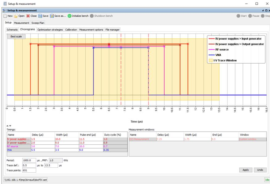
Figure 8:6 Example of Chronogram defined with the AMCAD PIV easy configurator
